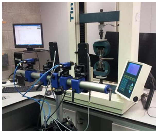
Figure 2. DIC camera and Tinius Olsen test machine. [Color figure can be viewed in the online issue, which is available at wileyonlinelibrary.com.]
